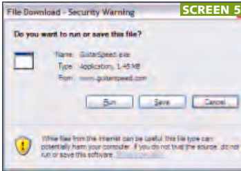
Windows saves the warning about running exe files from the Internet in an ADS
